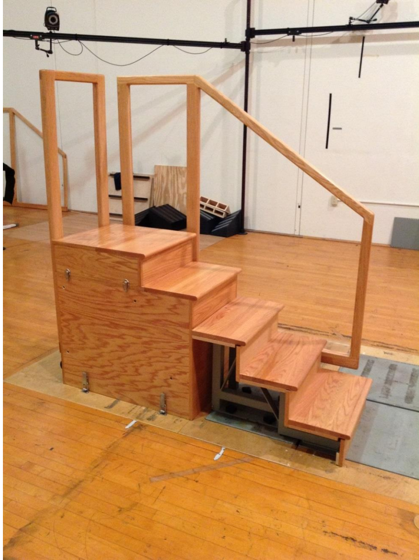
Figure 1. Complete setup of 5-step staircase for experimental data collections.
